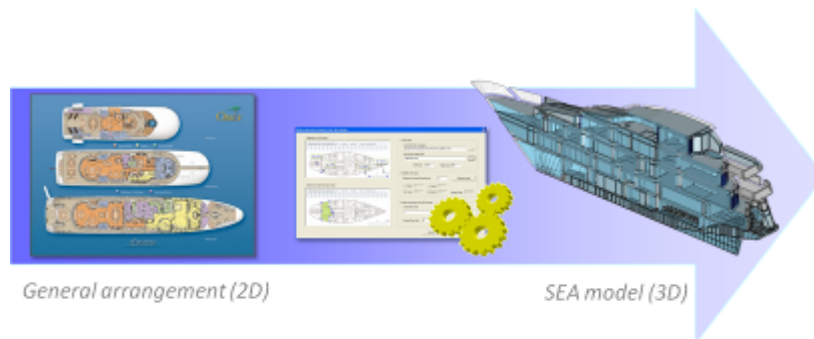
Figure 2: Model building process greatly simplified by automatic model building from 2D general arrangement drawings.
